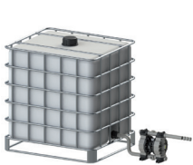
Pump installed below head (positive suction)
